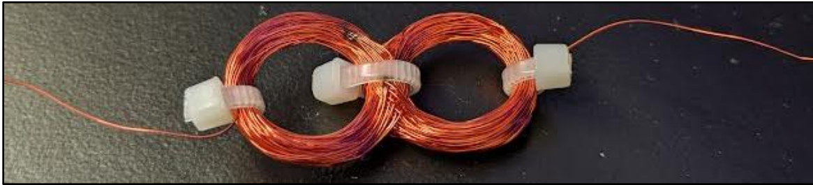
Figure 8.7 – Close-up of figure-eight coil showing burn mark
