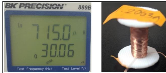
Figure 2.6 – Plastic spool coil and measured inductance
