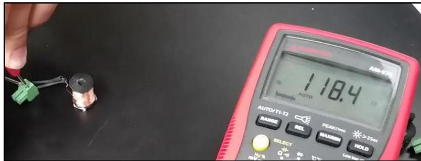
Figure 3.3 – Air core coil (118 \Omega and 87 mH). Max current flow is above 4 A (500 V/118 \Omega )
