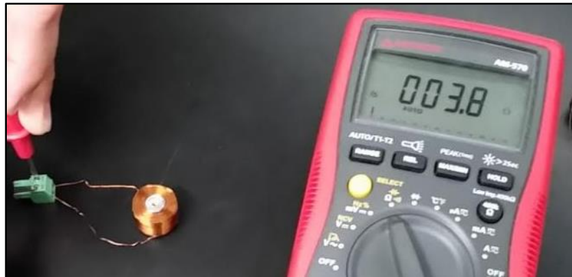
Figure 3.5 – Iron core coil ( 3.8 \Omega and 1.55 \text{ mH} ). Max current flow, MOSFET has 1 \Omega , is 100 \text{ A}
