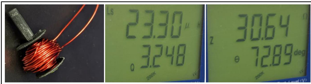
Figure 8.9 – Coil used for the interval robustness tests (insulating coating on magnet wire survived)
