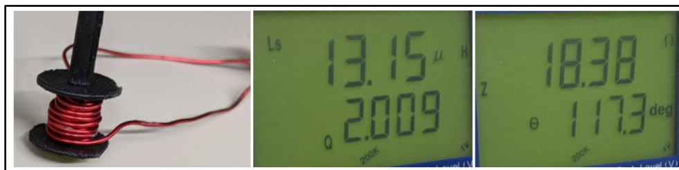
Figure 8.10 – Coil that burnt the IGBT when the circuit was charged to 1.2 kV and pulsed
