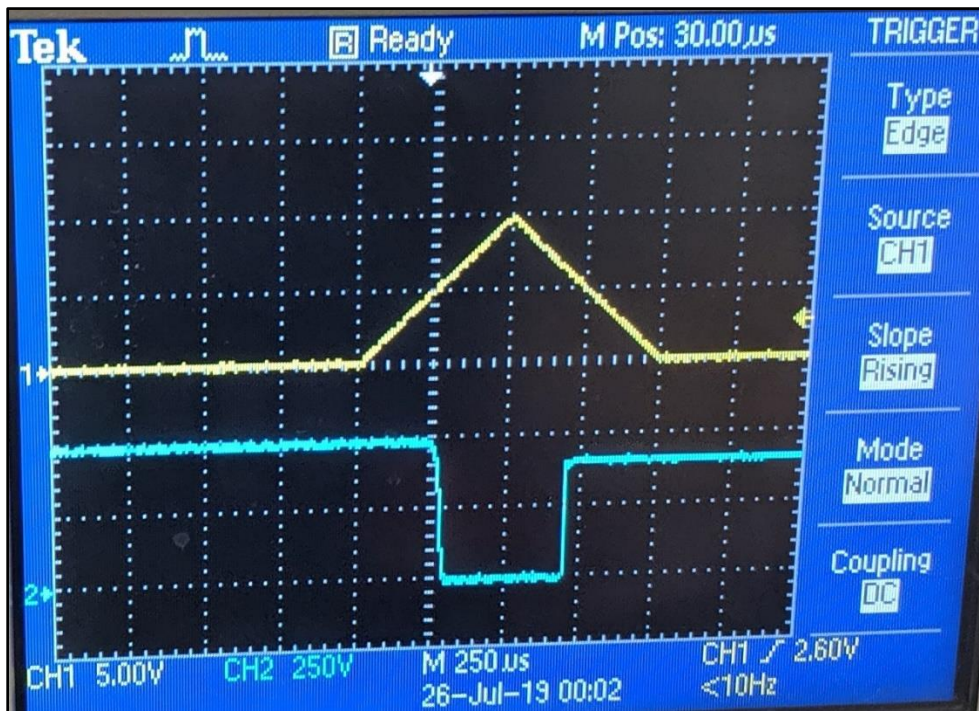
Figure 2.13 – Triangle wave input at 500V: (250 µs/div horizontal, and 250 V/div vertical)
