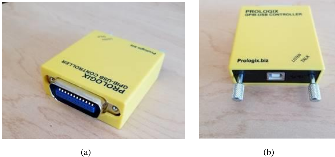
Figure 39 – Prologix GPIB-USB Controller (a) GPIB port (b) USB-B port
