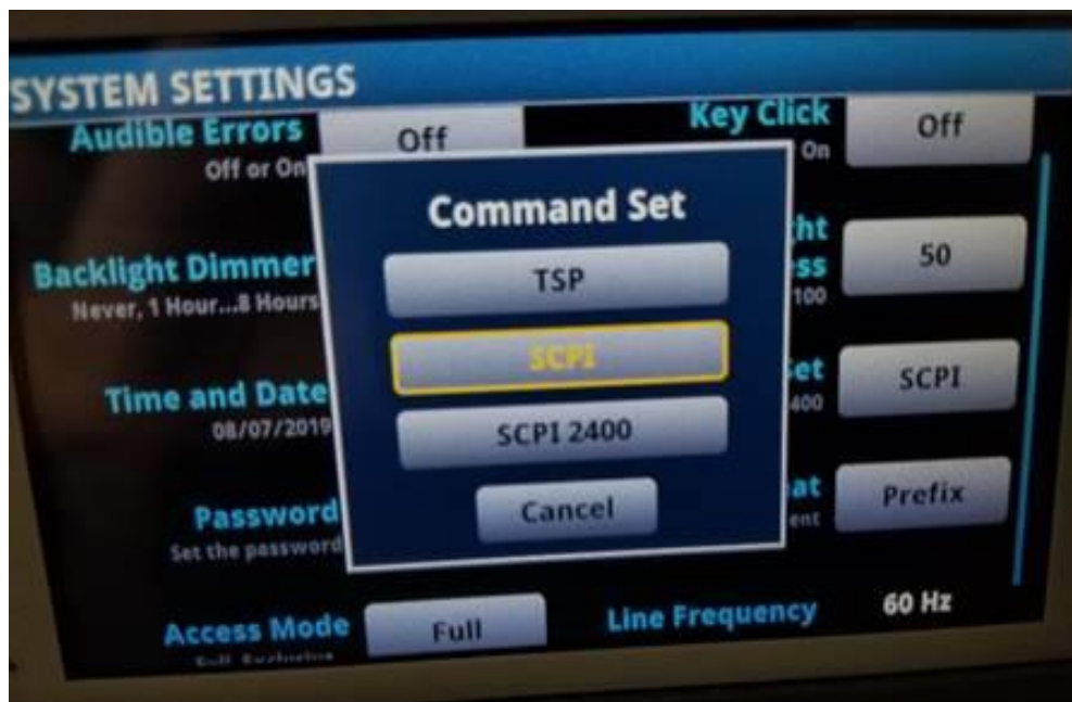
Figure 52 – Configuring Keithley with SCPI command set
