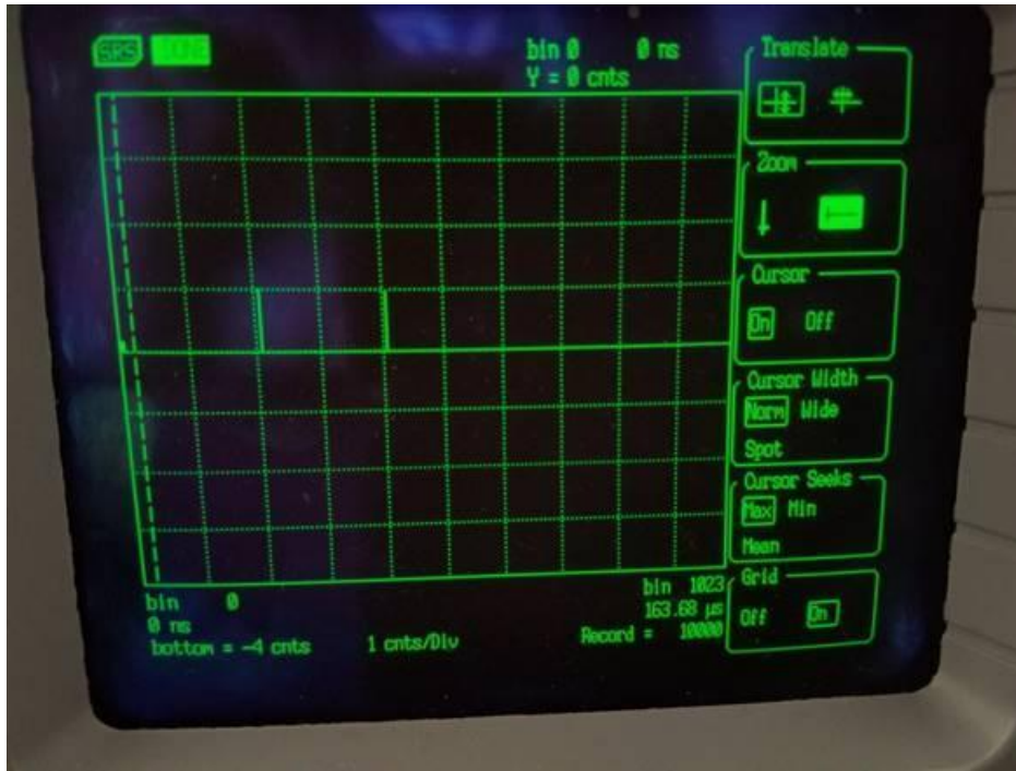
Figure 31 – Detecting pulses on the SR430
