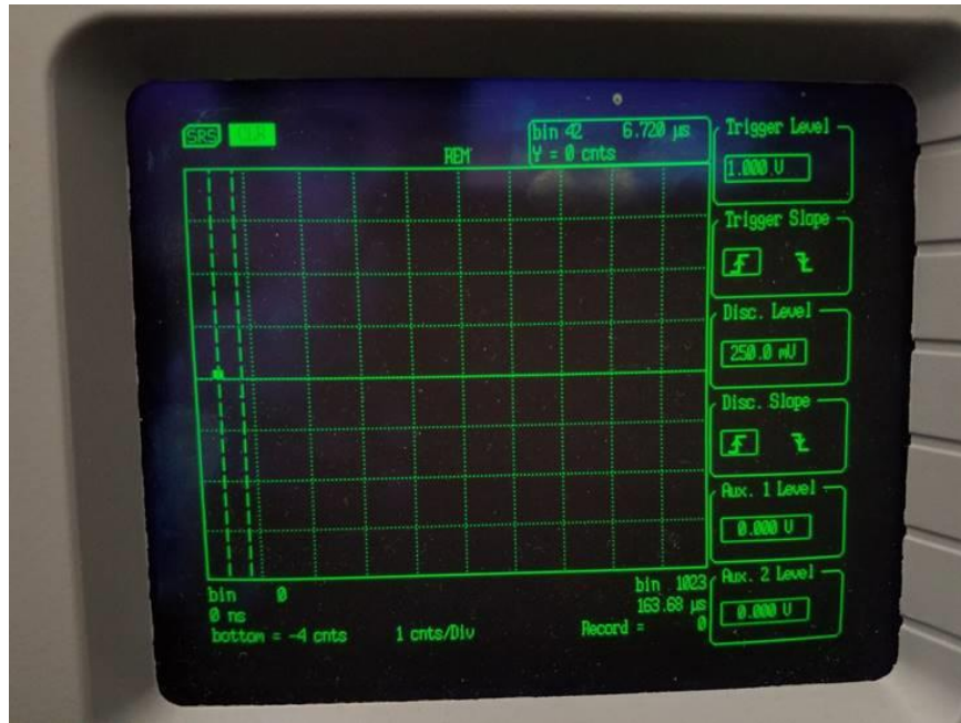
Figure 48 – SR430 Trigger level changed to 1V
