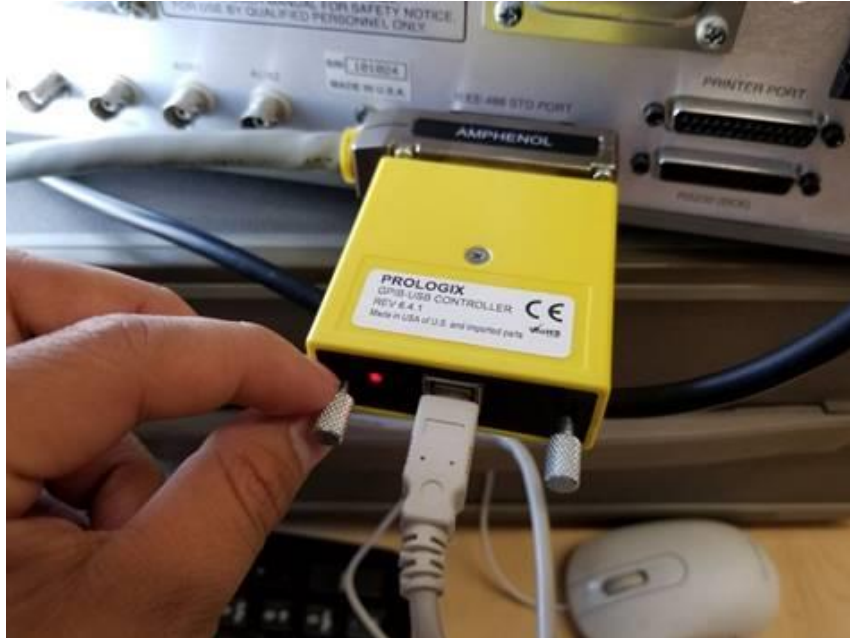
Figure 44 – Controller and GPIB device connected to bus
