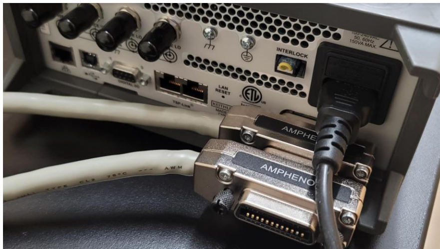
Figure 51 – GPIB connection to Keithley SourceMeter
