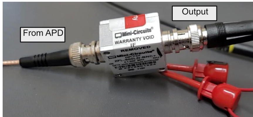
Figure 22 – Mini-Circuits ZFL-500LN-BNC+ Low Noise Amplifier (LNA)
