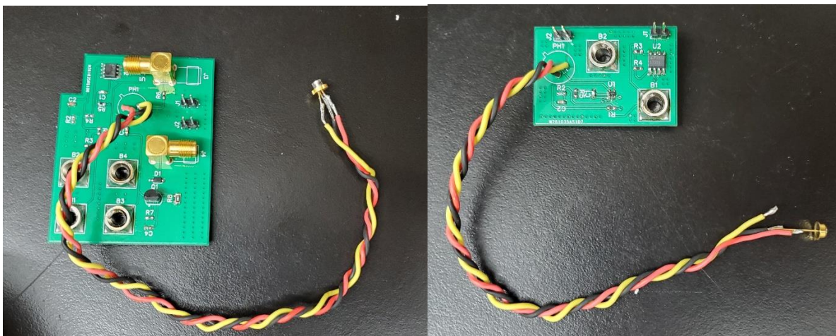
Figure 32 – Combinational and range finder PCBs
