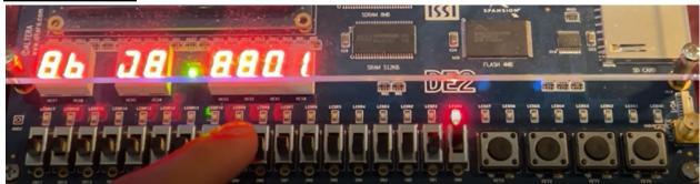
This is my Verilog code for the GDP that is implemented onto the DE2 board along with the 7 segment display. Here, the input is 1 and the output is 1.
