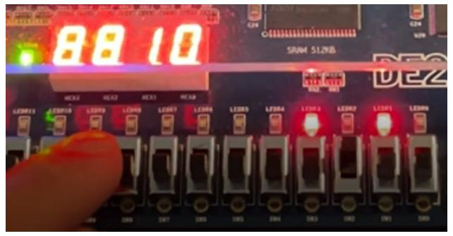
This is my Verilog code for the GDP that is implemented onto the DE2 board along with the 7 segment display. Here, the input is 4 and the output is 10.
