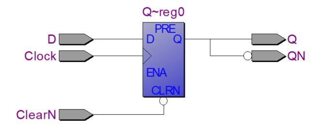
This is the RTL view for my D flip flop with asynchronous low clear and complementary output.
