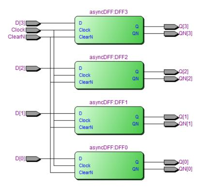
This is the RTL View of the structural 4-bit DFF register.
