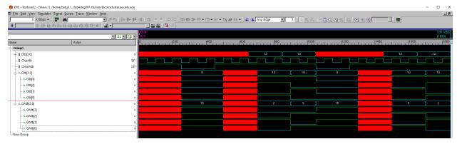
These are my VCS waveforms for the 4-bit DFF register. The blocks of red indicate delay or if the output is a "don't care (X) value".
