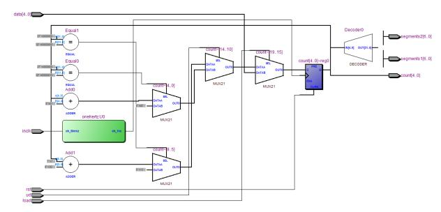
This is my RTL view for the 5-bit mod-25 up/down counter including a clock divider and a 7 segment display.
