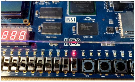
This is a picture of a DE2 board following an AND gate when the inputs are 1 and 1 leading to an output of 1 (on).
