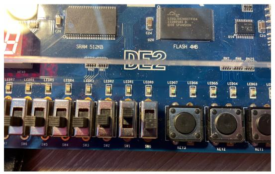
This is a picture of a DE2 board following an XNOR gate when the inputs are 1 and 0 leading to an output of 0 (off).
