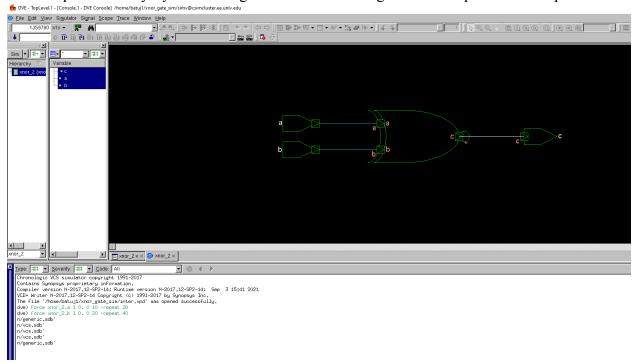
This is a picture of the schematic for my XNOR gate with 2 inputs and 1 output.
