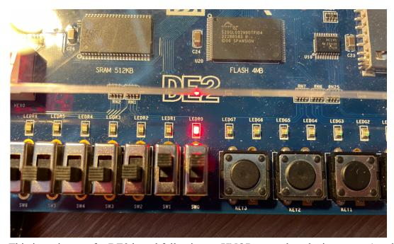
This is a picture of a DE2 board following an XNOR gate when the inputs are 1 and 1 leading to an output of 1 (on).
