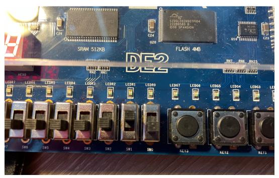
This is a picture of a DE2 board following an AND gate when the inputs are 1 and 0 leading to an output of 0 (off).
