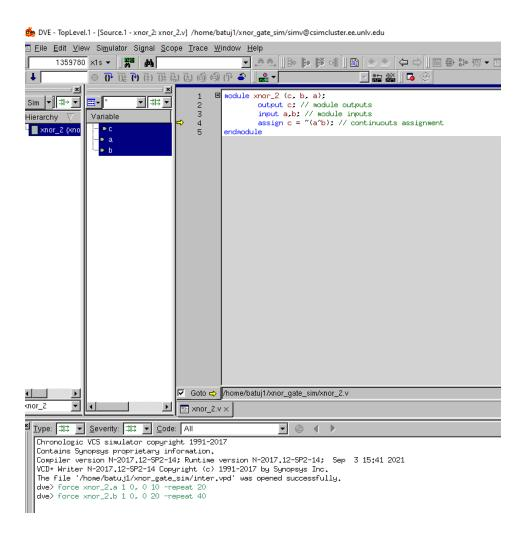
This is a picture of my SystemVerilog code for an XNOR gate with 2 inputs and 1 output.
