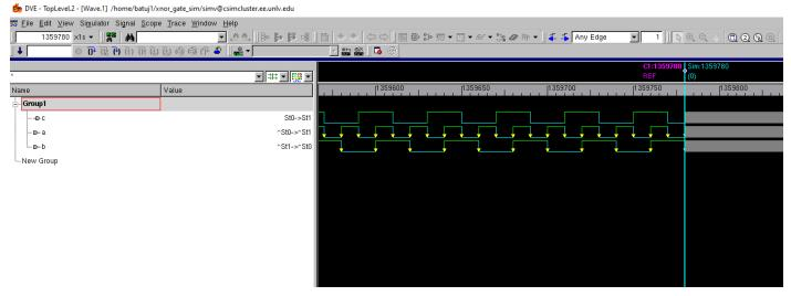
This is a picture of my XNOR waveforms in Synopsys indicating the combinational logic where the output would be 1 or 0.
