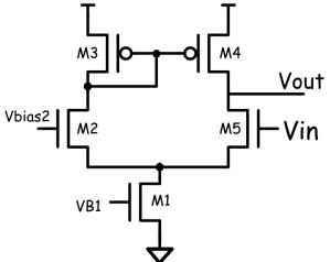
From the Diff-Amp TIA, a bias voltage was created for the diff-pair so that the input/output voltage can shift relative to the voltage at the other side of the gate.
