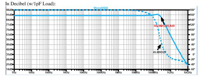
Looking at the above simulations, the bandwidth is choked down to 300MHz due to the 1pF capacitor load. The other thing to take into consideration is the phase of the output relative to the input signal, where the difference is well over 135°. Note that there is slight Q-peaking happening near the bandwidth cutoff, which means our TIA is approaching instability and oscillation.
