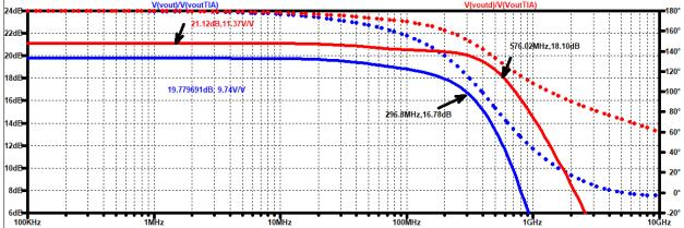
Although the overall voltage gain decreased from 11.37V/V to 9.74V/V, the source follower is able to carry the 1pF capacitive load!
