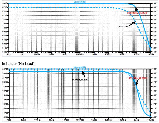
From the above, we see that the diff-amp TIA meets both the gain and bandwidth specification! However, what will indecisively dictate the TIA bandwidth is the load it needs to drive, seen in the next simulation.
