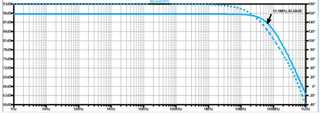
From the above, we see that the gain is high, however the circuit is only able to get up to 7MHz and this is due to the natural RC circuit that is achieved between the large resistance at M4 and 1pF capacitor. By estimation,
