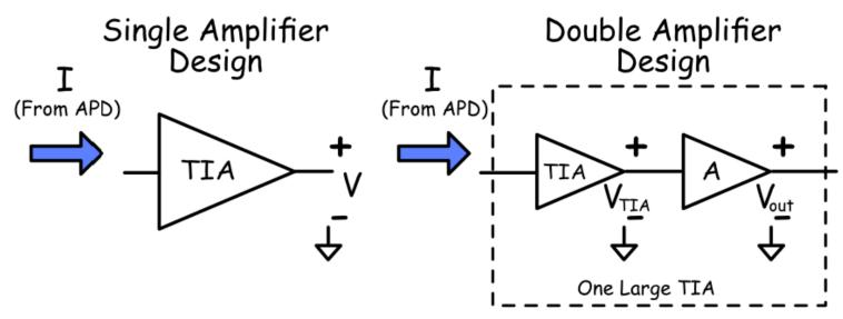
Note that in the above figure, a current will always be at the input stage of the amplifier, and the output stage will always be a voltage.
