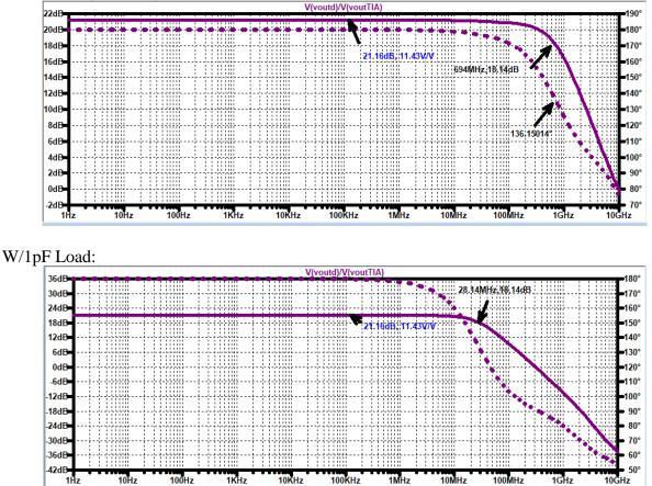
The voltage amplifier's maximum bandwidth is around 694MHz, however, adding the 1pF load bring the bandwidth down to nearly 30MHz!
