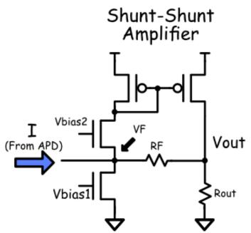
From above, the input current flows towards the feedback node and mixes with the feedback current, and the output is shunted towards the feedback node.
