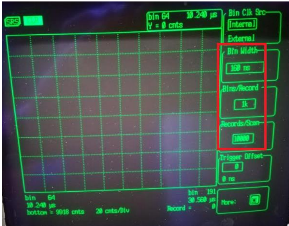
Figure 6.25 – SR430 Screen Displaying Bin Width, Bits per Record, and Records per Scan
