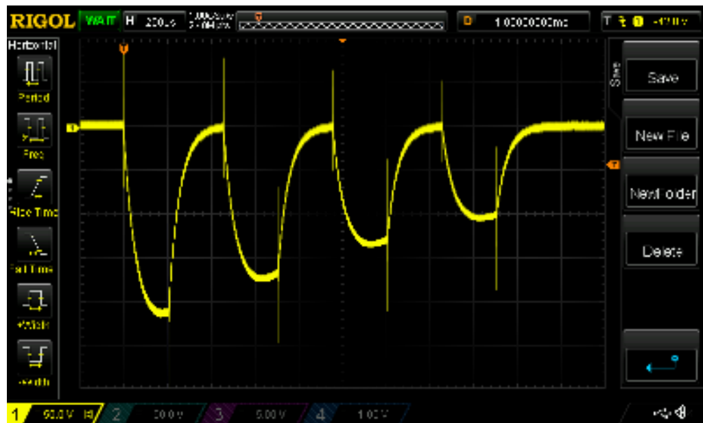
Figure 8 – Current through the coil showing 50 A/div and 200 \mu s/div.
