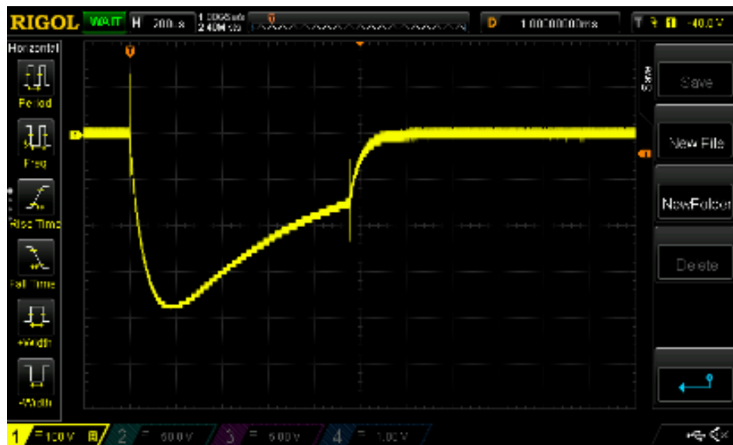
Figure 9 – Current through the coil when the power supply is increased to 1,200V. Scale is 100A/div and 200 \mu s/div.
