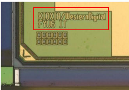
3D NAND Die Marking Photograph
