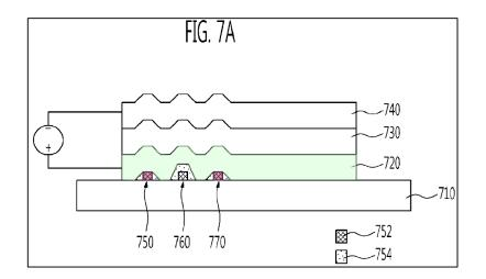
One problem with OLED's is that IR-drop that may occur due to resistance of components such as the anode and the cathode. *Id.*, [0009]. Han discloses a solution that includes the addition of "first and third subsidiary electrodes 750 and 770, which may be bonded to the anode 720 and function to reduce a resistance component of the anode 720." *Id.*, [0032]. Han further discloses that "each of the first and third subsidiary electrodes 750 and 770 may be electrically connected in
