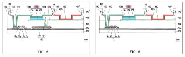
Further, there is also no complete overlap of the second auxiliary electrode 460 and the LED in the horizontal direction, because there is no overlap of the second auxiliary electrode 460 and the first electrode layer 132 in the horizontal direction. *Id.*
