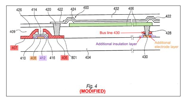
bus line 430 and anode 406 are electrically connected. EX1003, ¶130.
