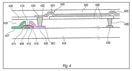
A POSITA would have understood that the a-Si layer 414 forms a channel layer for transistor 410. EX1003, ¶86. Transistors are active devices. EX1001, 3:33-59.
