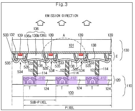
A POSITA would have understood that passivation layer 124 is made of insulating material, so that electrical features of TFT T are not electrically shorted together which would render the device in operatable. EX1003, ¶197.
