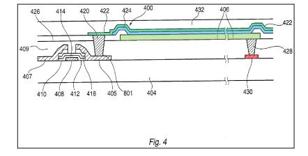
OLED 400 is considered "above" the bus line 430 because a portion (but not all) of OLED 400 vertically overlaps with bus line 430, in the same way that a portion (but not all) of light emitting device 130 vertically overlaps with first auxiliary electrode 120 for the embodiments of the 509 patent. EX1001, Figs. 2-5. EX1003, ¶96.
