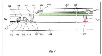
Alternately, bus line 430 could be connected in parallel to just a portion of the anode 406, which would still result in bus line 430 serving as a supplemental electrode to reduce the total resistance of the pixel structure. EX1003, ¶227.
