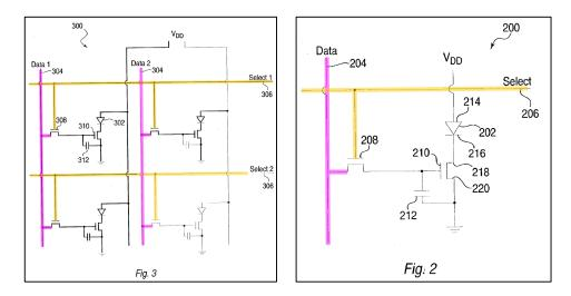
A voltage applied to the select line 306 will turn on transistor 308. *Id.*, Fig. 3, [0017]. In comparing Fig. 1 of the 509 patent and Fig. 2 of Weaver, the line configurations of the circuit designs are essentially identical in both configuration and function. EX1003, ¶82.
