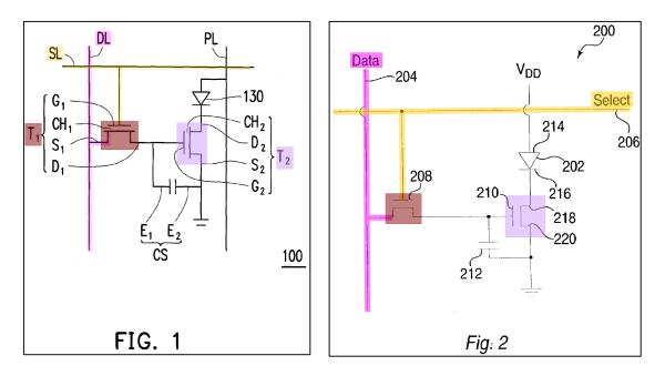
The active device (transistor 210/310/410) includes a gate 408, an a-Si layer 414, a source 220, 405, and a drain 218, 407. *Id.*, [0019], [0024], Fig. 2-4.
