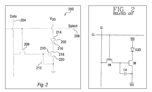
A POSITA would have understood the problem involved, namely that higher resistance between the power or ground line to the light emitting device would consume more power and require higher operating voltages, and can require larger wiring widths in order to achieve a desired performance. *Id.*, ¶128; EX1005,
