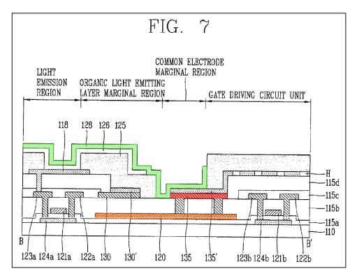
A light emitting device includes electrode 118 as an anode, an organic light emitting layer 126 on electrode 118, and electrode 128 as a cathode on the organic light emitting layer 126. EX1005, [0081], [0089], [0091], Fig. 7. Lee053 discloses a first auxiliary electrode having a top electrode layer (second power wiring 135) and a bottom electrode layer (dummy wiring 120), which is made of
