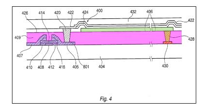
Weaver discloses that via holes 428 are formed in the passivation layer to the bus line 430, and metal plugs are formed therein (to electrically connect bus line 430 to anode 406). EX1004, [0035], Fig. 4.
