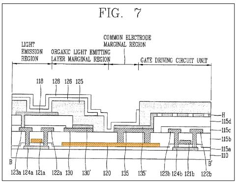
Lee053 discloses that the first gate electrode 121a is included in "gate wiring." *Id.*, [0071]. Lee053 also discloses that the dummy wiring 120 is "made of the metal for a gate wiring." *Id.*, [0073]. The first gate electrode 121a and the dummy wiring 120 are both formed on layer 115a. *Id.*, Fig. 7. Therefore, Lee053 discloses or at least renders obvious that the dummy wiring 120 and the first gate electrode 121a of the TFT active device belong to the same layer. EX1003, ¶134.
