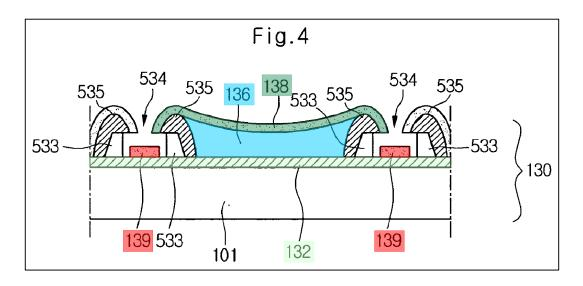
Bae discloses that auxiliary electrodes 139 is an electrode that is supplemental to other electrodes in the structure, and is a supplemental electrode that reduces the total resistance of the pixel structure." EX1003, ¶196.
