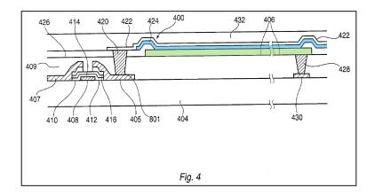
Organic layer 424 emits light when sufficient current is passed between the anode 406 and cathode 422. *Id.*, [0027].
