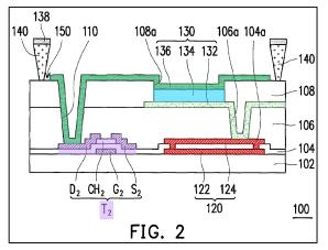
The first auxiliary electrode 120 includes a bottom electrode layer 122 and a top electrode layer 124. *Id.*, 4:6-8; Fig. 2. In another embodiment, the first auxiliary electrode 120 includes only a bottom electrode layer 222. *Id.*, 6:29-34; Fig. 3.
