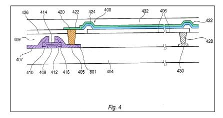
Cathode 422 is electrically connected to the source region 405 of transistor 410 by a metal plug filling via 420. *Id.*, [0025], Fig. 4.
