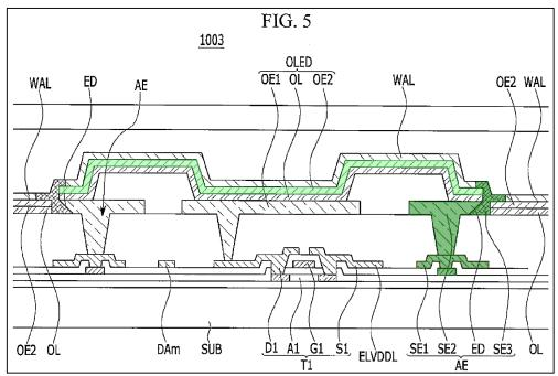
The first auxiliary electrode portion SE1, the second auxiliary electrode portion SE2 and the third auxiliary electrode portion SE3 (of auxiliary electrode AE) wholly thickens second electrode OE2 to reduce sheet resistance and voltage drop. *Id.*, [0098].
