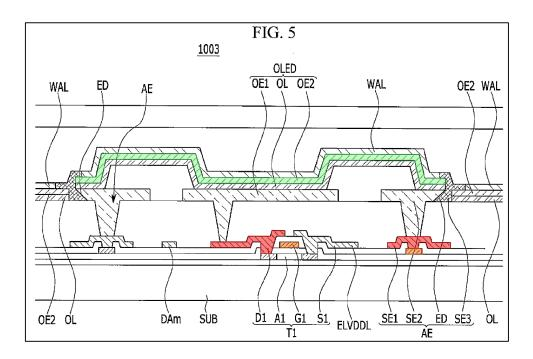
In combining the teachings of Weaver and Song as set forth above in §VII.A, it would have been obvious to a POSITA to form the top electrode layer of the first auxiliary electrode (i.e. bus line 430), and the source region 405 and the drain region 407 transistor 410 in Weaver, so they belong to the same layer. EX1003, ¶170; EX1004, [0034], Fig.4, Fig. 6.
