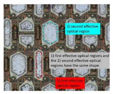
35. As shown below, in the pixels of the external display of the Motorola RAZR displayed at 500 times magnification and the external OLED panel of Motorola RAZR being illuminated, the 1) first and 2) second effective optical regions do have respective electronic circuits to drive the electro-optical elements 1') and 2') provided in the 1) first and 2) second effective optical regions.
