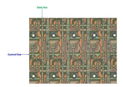
43. As shown below, in a pixel circuit of the external display of the Motorola RAZR after anode layer and source layer are removed and displayed at 1500x magnification, the external OLED panel has a first power line that has a first portion extending in a first direction and a second portion extending in a second direction that intersects the first direction.
