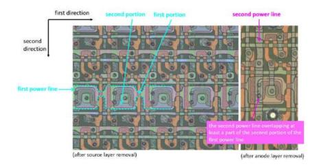
45. As shown below, in a pixel circuit of the external display of the Motorola RAZR after anode layer and source layer are removed and displayed at 1500x magnification, the external OLED panel has an inter-layer insulating film that is disposed between the first power line and the second power line.
