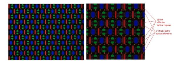
30. As shown below, in the pixels of the external display of the Motorola RAZR displayed at 500 times magnification, the external OLED panel has a plurality of 2) second effective optical regions provided above the substrate, and 2') second electrooptical elements are provided in the 2) second effective optical regions.
