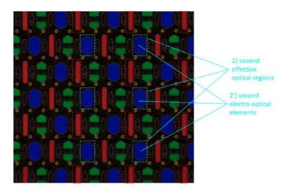
31. As shown below, in the pixels of the external display of the Motorola
