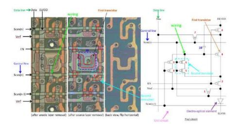
50. As shown below, in a pixel circuit of the external display of the Motorola RAZR after anode layer are removed and in a back view of a pixel circuit of the external display of the Motorola RAZR both displayed at 1500x magnification, in the unit circuit of the external OLED panel, the wiring is formed in a layer which is different from a layer in which the first semiconductor film and the second semiconductor film are formed.
