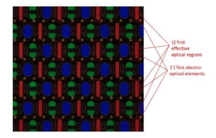
34. As shown below, in the pixels of the external display of the Motorola RAZR displayed the external OLED panel of Motorola RAZR, the 1) first effective optical regions and the 2) second effective optical regions have the same shape.
