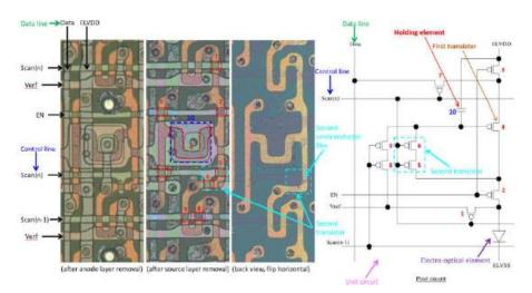
49. As shown below, in a pixel circuit of the external display of the Motorola RAZR after anode layer is removed and displayed at 1500x magnification, the unit circuit of the external OLED panel has a wiring connected between the second transistor and the gate of the first transistor, and the first transistor supplying a current based on the gate voltage to the electro-optical element.
