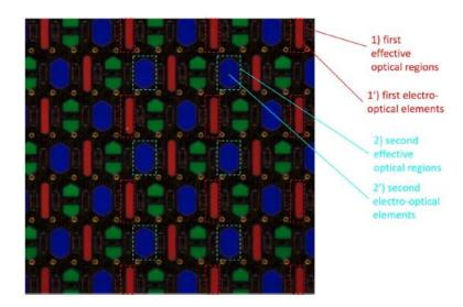
38. As shown below, in the pixels of the external display of the Motorola RAZR displayed at 500 times magnification and the external OLED panel of Motorola RAZR being illuminated, each of the 1') first electro-optical elements and the 2') second electro-optical elements is an electroluminescent element. The external OLED panel has a first electrode, a second electrode, and a light emission layer that is disposed between the first electrode and the second electrode.
