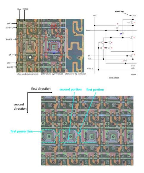
44. As shown below, in a pixel circuit of the external display of the Motorola RAZR after anode layer is removed and displayed at 1500x magnification, the external OLED panel has a second power line that extends in the second direction, the second power line overlapping at least a part of the second portion of the first power line.
