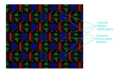
41. As shown below, in the pixels of the external display of the Motorola RAZR displayed at 500 times magnification, in the external OLED panel of Motorola RAZR, each of the 1) first effective optical regions in which the 1') first electro-optical elements are provided being arranged at regular intervals in a 8) column and 9) row directions of a display area.
