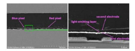
39. As shown below, in the pixels of the external display of the Motorola RAZR displayed at 500 times magnification and the external OLED panel of Motorola RAZR being illuminated, the 1') first electro-optical element has a light-emitting layer that includes organic material so as to emit red light, and the 2') second electro-optical element has a light-emitting layer that includes organic material so as to emit blue light.
