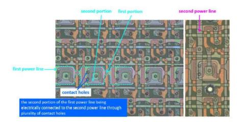
47. As shown below, in a pixel circuit of the external display of the Motorola RAZR after anode layer are removed and in a pixel circuit of the external display of the Motorola RAZR after source layer are removed and displayed at 1500x magnification, the unit circuit of the external OLED panel has a second transistor that includes a second
