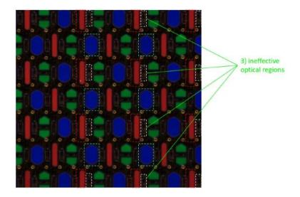
32. As shown below, in the pixels of the external display of the Motorola RAZR displayed at 500 times magnification, the external OLED panel of Motorola RAZR, each of the whole 3) ineffective optical regions is arranged so as to be 4) sandwiched by two of the first effective optical regions and so as to be 5) sandwiched by two of the second effective optical regions.
