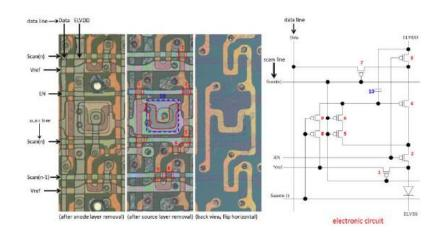
36. As shown below, in a pixel circuit of the external display of the Motorola RAZR, the external OLED panel of Motorola RAZR, there are pixels provided so as to correspond to respective intersections of a plurality of 6) scan lines and a plurality of 7) data lines, the electronic circuits drive the electro-optical elements 1') and 2') in accordance with scan signals from the 6) scan lines and data signals from the 7) data lines.
