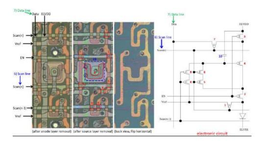
37. As shown below, in the pixels of the external display of the Motorola RAZR displayed at 500 times magnification and the external OLED panel of Motorola RAZR being illuminated, the 1') first electro-optical element (red) and 2') the second electro-optical element (blue) include two electro-optical elements selected from an electro-optical element that emits green, an electro-optical element that emits blue, and an electro-optical element that emits red.
