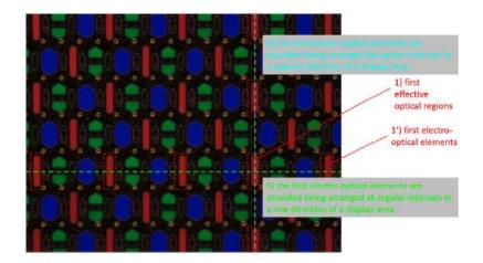
42. As shown below, in a pixel circuit of the external display of the Motorola RAZR after anode layer removed and displayed at 1500x magnification, the external OLED panel of Motorola RAZR has a data line and a control line.
