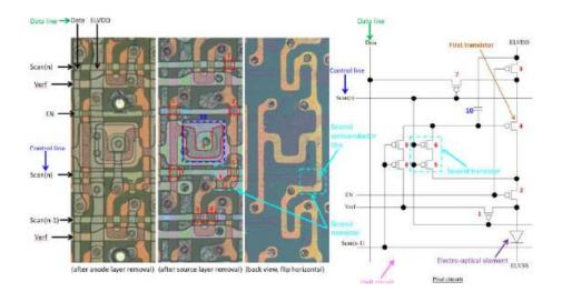
48. As shown below, in a pixel circuit of the external display of the Motorola RAZR after anode layer are removed and in a pixel circuit of the external display of the Motorola RAZR after source layer are removed and displayed at 1500x magnification, the unit circuit of the external OLED panel has a holding element that is connected to the gate of the first transistor and holds a gate voltage of the first transistor according to a data signal.
