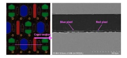
40. As shown below, in the pixels of the external display of the Motorola RAZR displayed at 500 times magnification, in the external OLED panel of Motorola RAZR, 2) the second effective optical regions are not arranged so as to be adjacent to each other.
