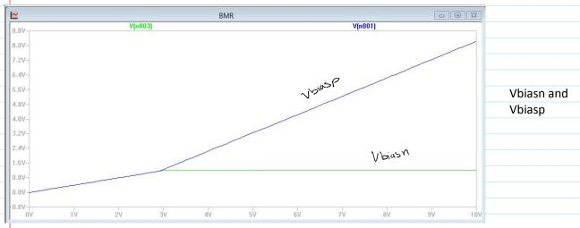
From the figure above, we can see that Vbiasn stays constant after the minimum VDD voltage (~3V) and Vbiasp follows VDD after that same minimum VDD voltage.
