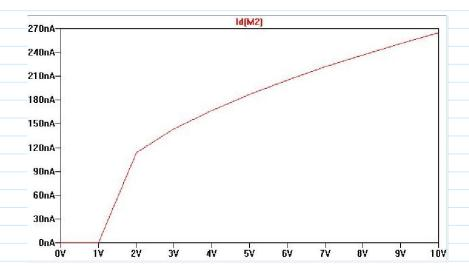
We can see that our BMR from simulations rounds out at around 180-250nA. One of the possible reasons for this may be because that we are using a resistor as a startup and the resistor will steal some current form the mirror.
