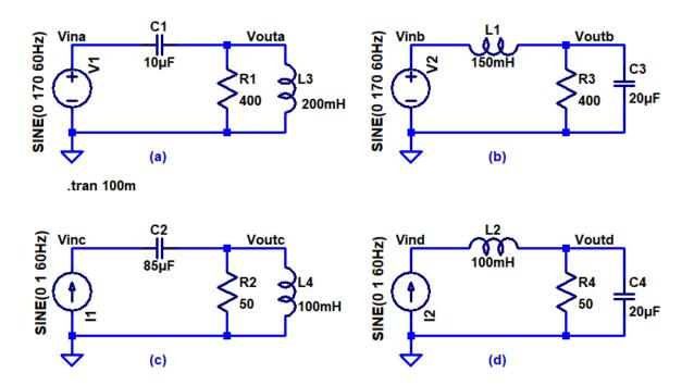
2. Determine the frequency response (Vout/Vin, both magnitude and phase) of the circuits in problem 1. Verify your hand calculations and plots using LTspice. (1 point each)
