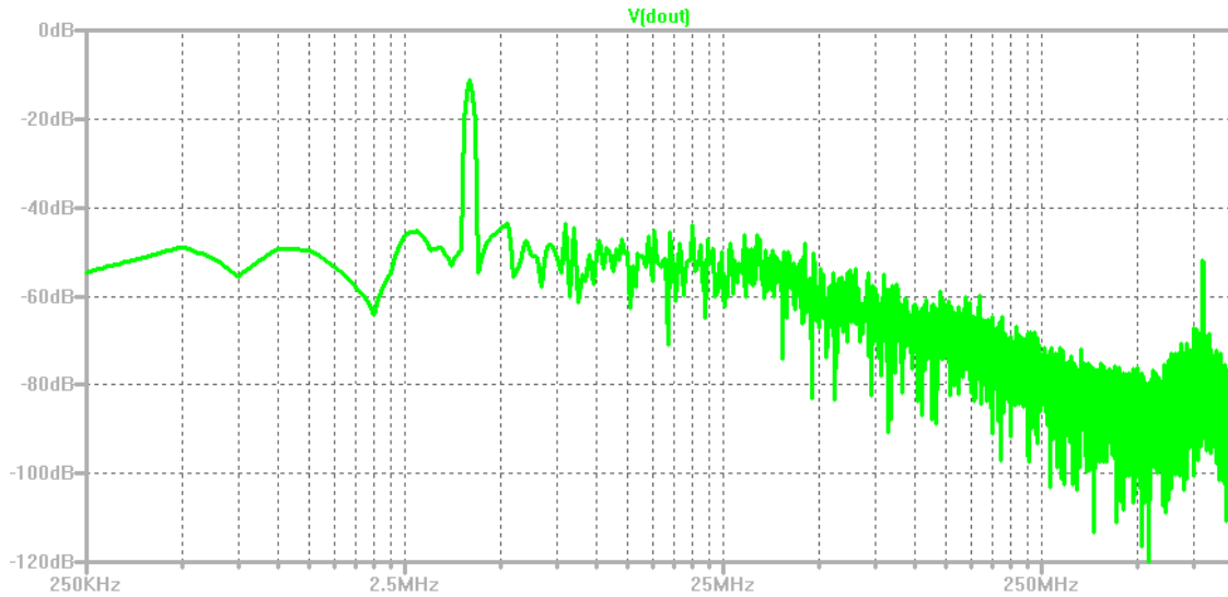
Figure 3. The FFT plot for the filtered output data (log frequency)
