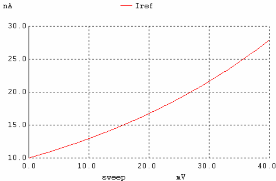
Figure 1: WinSpice simulation results for Beta multiplier with threshold voltage mismatch form 0 to 40 mV.
