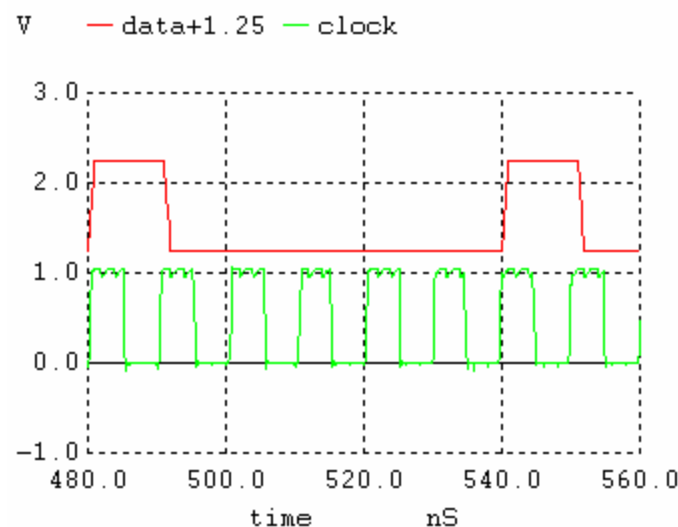
Figure 1 DPLL with passive loop filter, noise on VDD causes loop not to lock.
