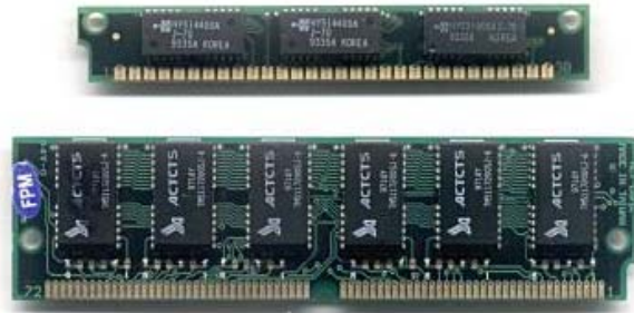
From top to bottom: SIMM (30-pin), SIMM (72-pin) [5]
