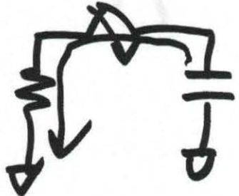
Figure 10.2 Diagram used to determine average resistance of a MOSFET during switching.
