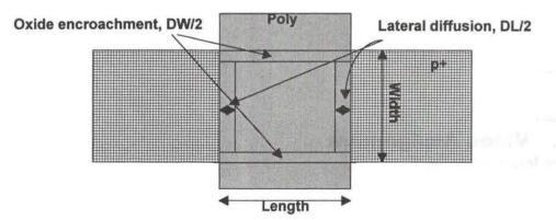
**Problem 4.5**: See figure above. (a) From the BSIM model parameters for the p-channel MOSFET in appendix A, DL (dl) = 0.84424 um. (b) The lateral diffusion does not affect the width of the MOSFET. From the above layout, the location of the lateral diffusion can illustrate this clearly.
