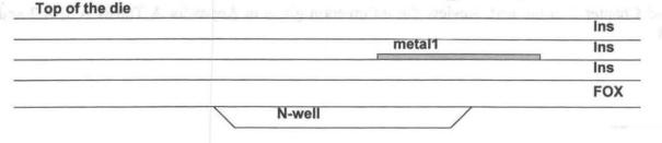
**Problem 3.6**: Considering only the plate capacitance, assume the area of metal1 and metal2 is A um<sup>2</sup>. The capacitance between metal1 and metal2, from App. A, is 38 aF/um<sup>2</sup>. The capacitance between metal1 and substrate is 26 aF/um<sup>2</sup>. The voltage change on metal1 =  $1V \times (38AaF/\mu m^2/(38A + 26A)aF/\mu m^2) = 0.594V$ .
