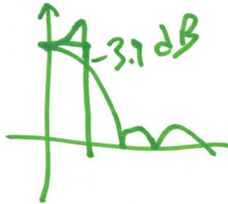
Figure 3.35 Second-order lowpass filter.
