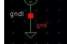
, you should NOT also use a Stimuli (Global source) since the result is two voltage sources connected to the same node (which will result in error and the simulation not running!).
