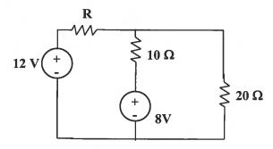
Removing the 10 ohm resistor and solving for the Thevenin Circuit results in:
