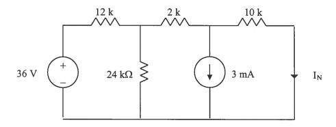
We can use superposition theorem to find  $I_N$ . Let  $I_N = I_1 + I_2$ , where  $I_1$  and  $I_2$  are due to 16-V and 3-mA sources respectively. We find  $I_1$  using the circuit below.
