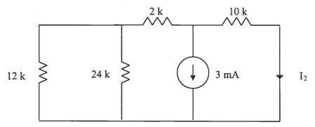
$$\begin{array}{l} 2k + 12k//24 \; k \; = 10 \; k\Omega \\ I_2 \! = \! 0.5 (\text{-3mA}) = \text{-1.5 mA} \\ I_N = 1.2 \, \text{-1.5} = \text{-0.3 mA} \end{array}$$
