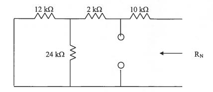
$R_{eq} = 10 + 2 + (12/\!/24) = 12 + 8 = 20 \ k\Omega$   $I_N$  is obtained from the circuit below.
