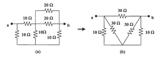
20||20 = 10 ohms. Transform the wye sub-network to a delta as shown in Fig. (b). 10||30 = 7.5 ohms.  $R_{Th} = R_{ab} = 30||(7.5 + 7.5) = 10$  ohms.
