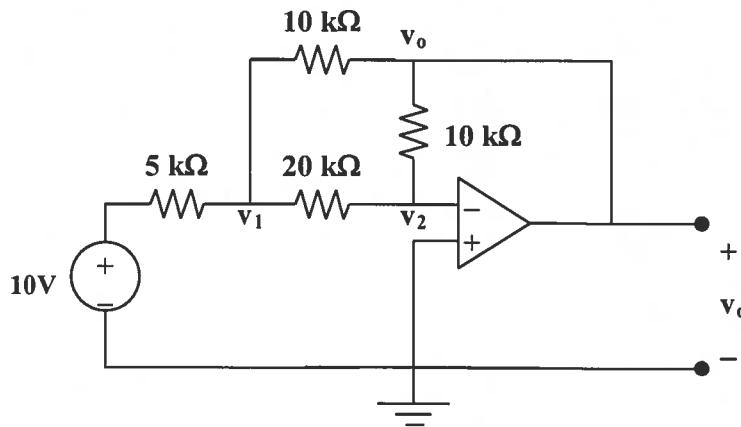
$$\text{But } v_2 = 0. \text{ Hence } 40 - 4v_1 = v_1 + 2v_1 - 2v_o \rightarrow 40 = 7v_1 - 2v_o \quad (1)$$
