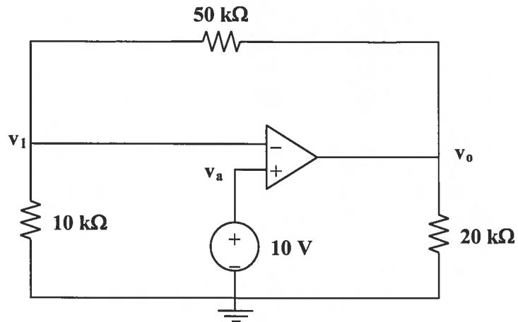
$$\text{At node 1, } \frac{0 - v_1}{10k} = \frac{v_1 - v_o}{50k}$$
