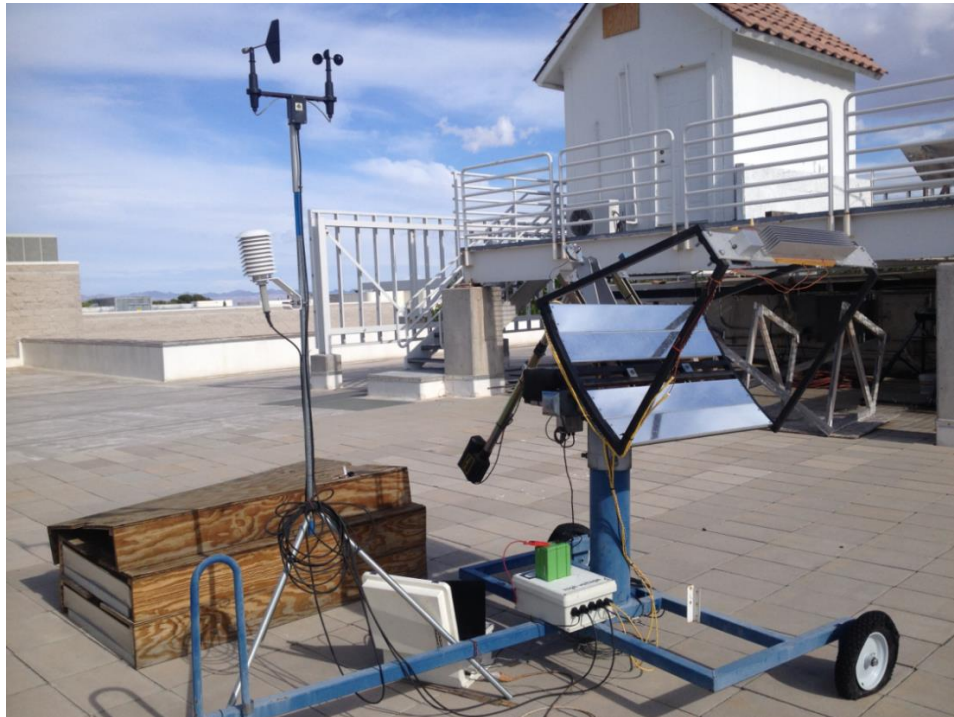
Figure 31 – Complete STEG energy-harvesting system
