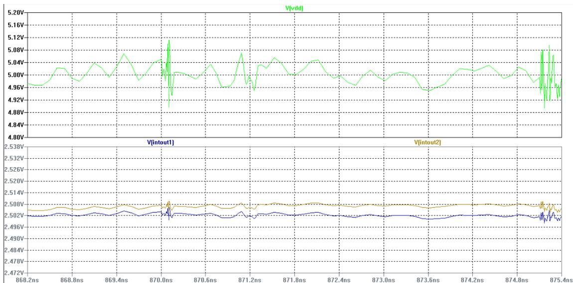
Figure 56: 50mV,RMS Supply Voltage Noise Affects Integrator Nodes
