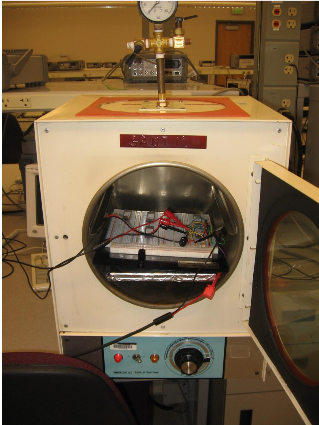
Figure 6.7 Temperature chamber used for testing DSM temperature sensors.
