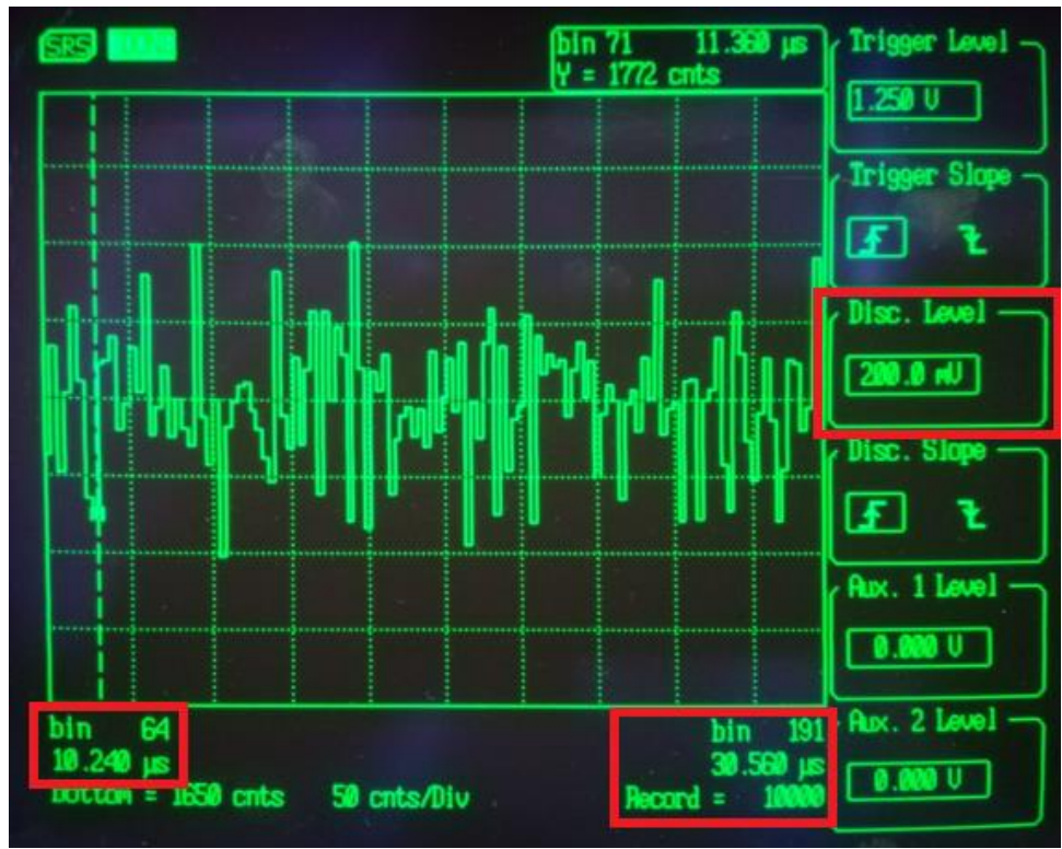
Figure 6.21 – SR430 Screen Displaying 200mV Discriminator Level, Bin 64 at 10.24μs, and Bin 191 at 30.56μs
