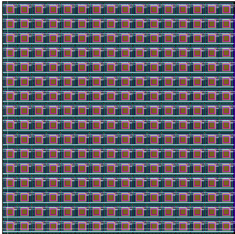
Figure 5.9 – Cadence Layout of SiPM Array (16x16 Array of SiPM pixels)
