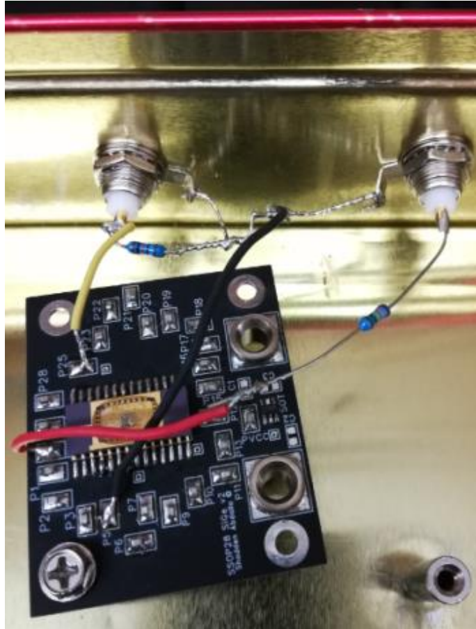
Figure 6.23 – Dark Box Connection of an APD in an SOIC-28 Package for DCR Tests
