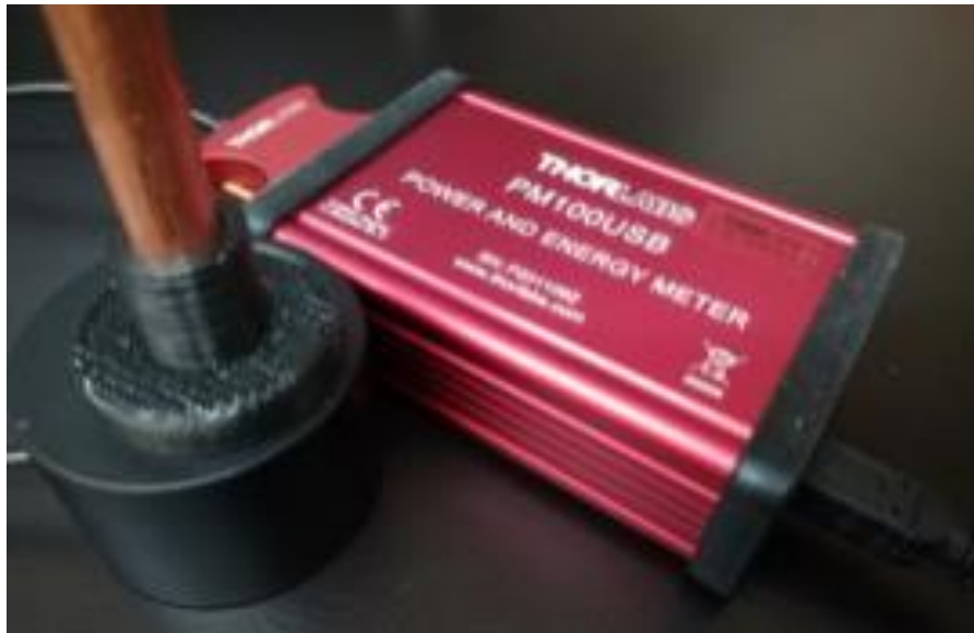
Figure 6.29 – Copper Tube Connected to Power Meter using Component 2a (shown), 2b, and 2c
