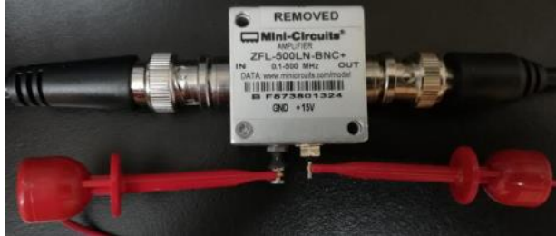
Figure 6.8 – Mini-Circuits ZFL-500LN-BNC+ Small Signal, Low Noise Amplifier (LNA) with a gain of 24dB
