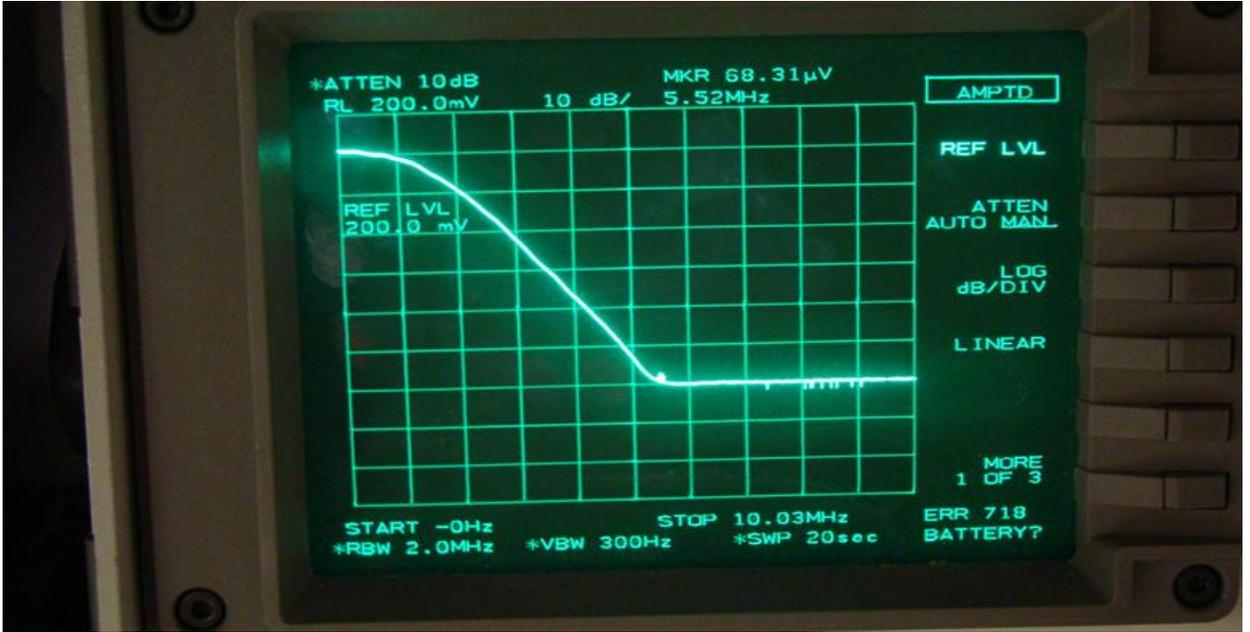
Figure 66. Spectrum analyzer output noise measurement of the improved TIA.
