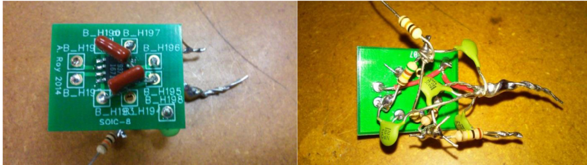
Figure 3.2 – Top and bottom of circuit on SOIC-8 breakout board.
