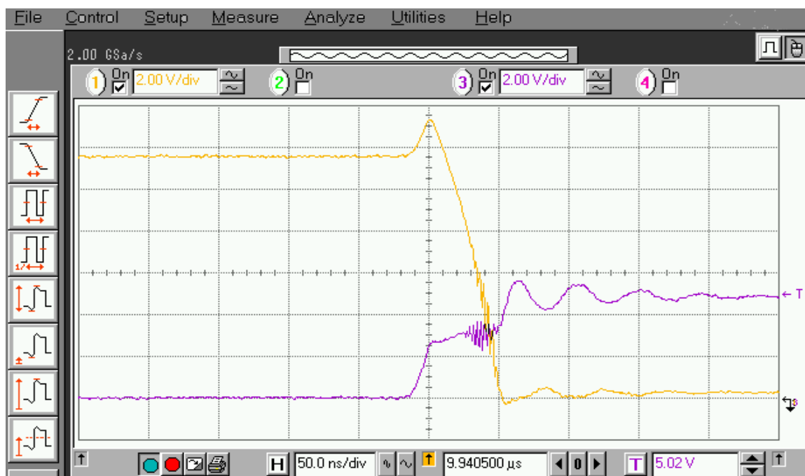
Figure 3.9: Fall time of the inverter measured on the PCB [20ns]
