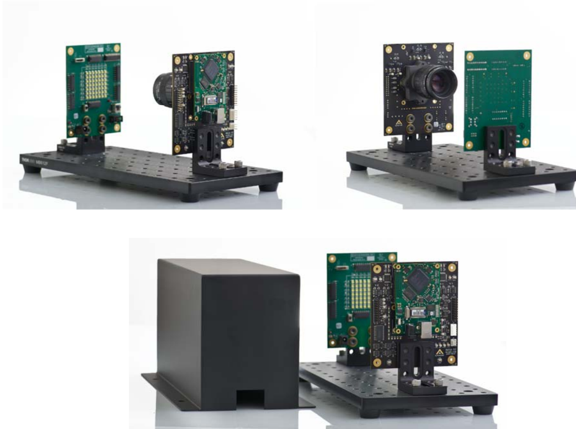
Figure 49: Test setup for measuring exposure and frame speed
