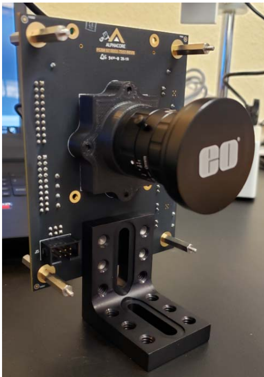
Figure 36: The camera PCB with the lens mount, the FPGA and the lens attached
