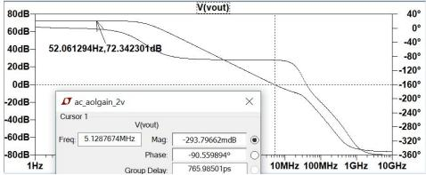
Gain of 72dB with a phase margin of 90 degrees. The gain and phase margin also stay the same at varying temperature.
