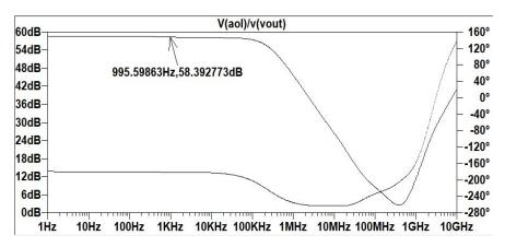
At higher frequencies, the PSRR is still at 58dB before dropping, whereas for the PSRR plus, the signal falls earlier, before 1kHz. Because of the compensation capacitor, at higher frequencies the ground noise contributions to the output signal decrease.
