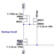
when some of them are at VDD, and MSU1 turns off, the other two transistors will be on, and send current into the gates of the transistors that have gone to ground and turn them back on. Once the current is stable, MSU3 turns on.
