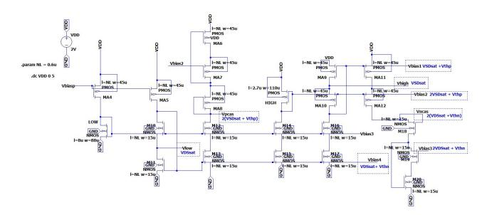
**Folded Cascode Topology:** This topology is best when generating bias voltages. This is because the method of diode-connecting the NMOS devices allows the PMOS current source to set the gate potentials of the NMOS current source that is diode connected beneath the two PMOS devices. This way, we can connect the currents and allow them to be at the same potential between the two sources. Current stealing is used with these connections.
