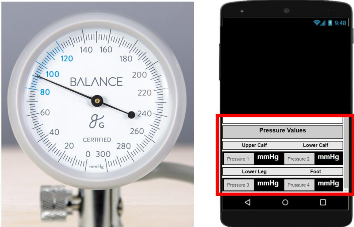
Figure 2.2 Mechanical Pressure Gauge and Smartphone Interface for Pressure Readings
