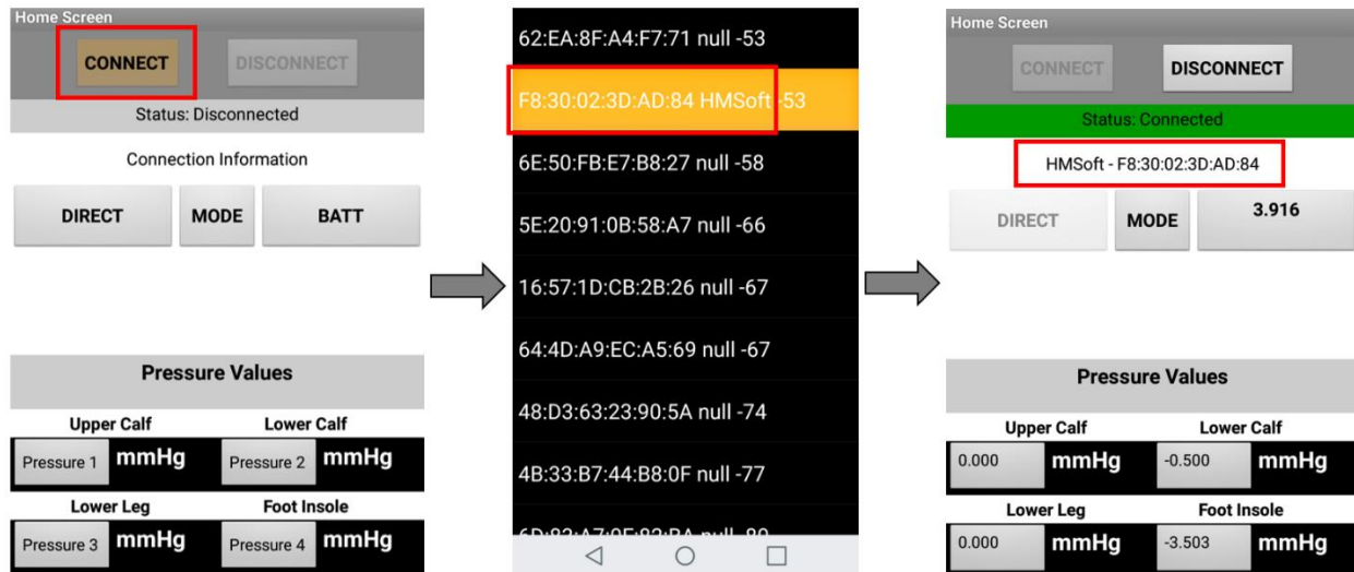
Figure 5.4 Connecting to a Device Using CONNECT Button and Device List
