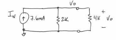
$$V_0 = 7.6 \text{ mA} \left(\frac{2 \text{ k}}{6 \text{ k}}\right). \text{ Yk}$$
