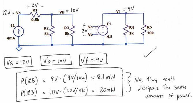
7. Determine each of the voltages labeled in the circuit below (Va, Vb, Vc, Vd) using mesh analysis. Do R2 and R3 dissipate the same amount of power? Show your power calculations to support your answer. (10 points)
