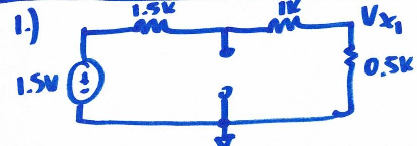
$$V_{x_1} = 1.5V \left( \frac{0.5k}{2.5k + 0.5k} \right) = 1.5V \left( \frac{1}{6} \right)$$
