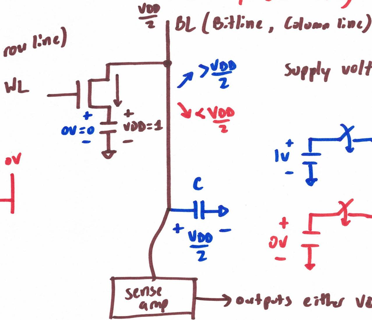
Supply voltage =  $V_{DD}$
