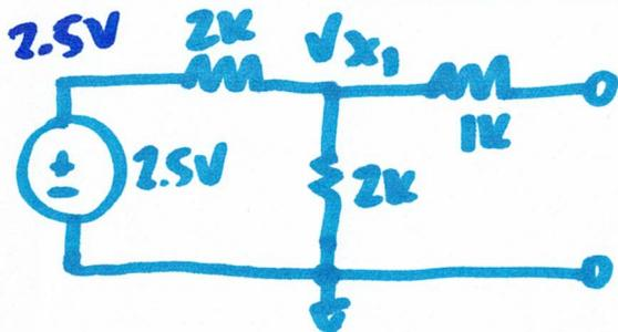
$$V_{x_1} = 2.5V \cdot \frac{2k}{4k} = 1.25V = V_{x_1}$$
