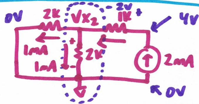
$$V_{x_2} = 1mA \cdot 2k = 2V = V_{x_2}$$
