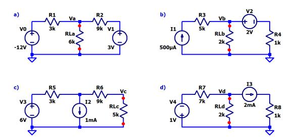
2. Determine the voltages and currents in the circuits given below using **both mesh analysis** and superposition. Verify your work using LTspice. No need to verify twice, but there should be hand calculations for both mesh analysis and superposition. (10 points)
