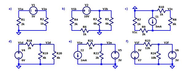
2. Determine the voltages labeled in the circuit below. Verify your work using LTspice. (3 points)
