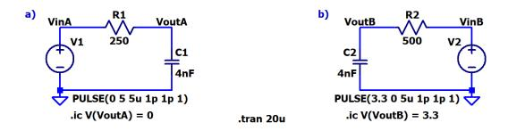
2. Repeat problem 1 for **Vi, Vx, and Vo** in the following RC circuit. Verify that your waveform sketches are correct using LTspice. (4 points)
