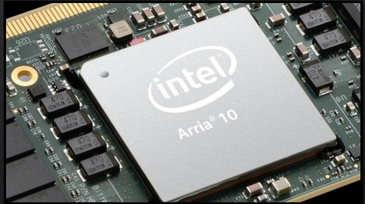
Figure 2: Intel Arria 10 FPGA soldered to a PCB. Source: [11]
