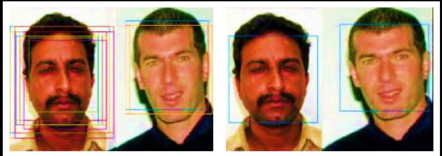
Figure 10: Example Image Showing Redundancy (left) and Removal of Redundancy (right) [6]
