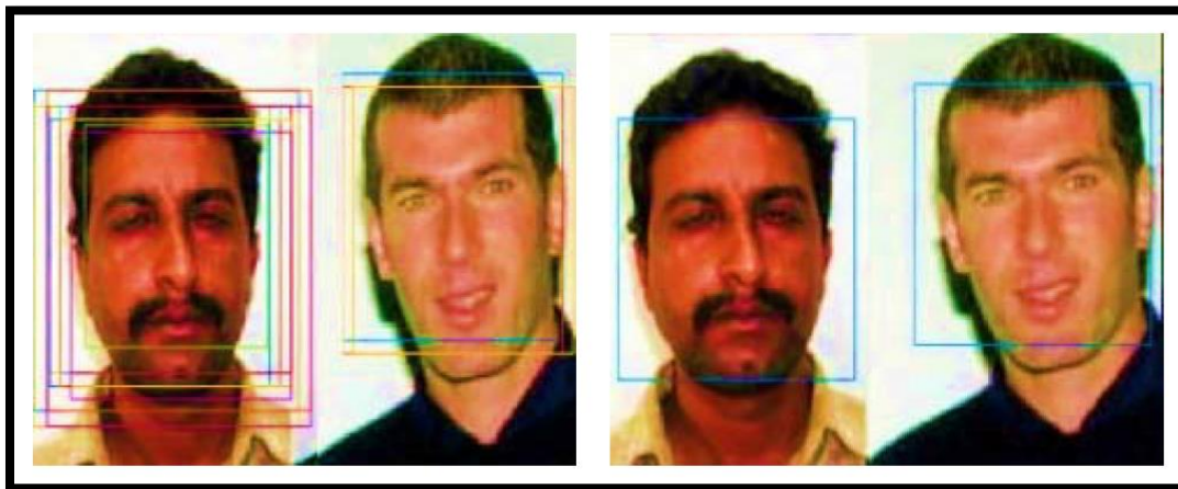
Figure 9: Redundancy Issue in Viola-Jones (left) Contrasted with No Redundancy Issue (right) [2]
