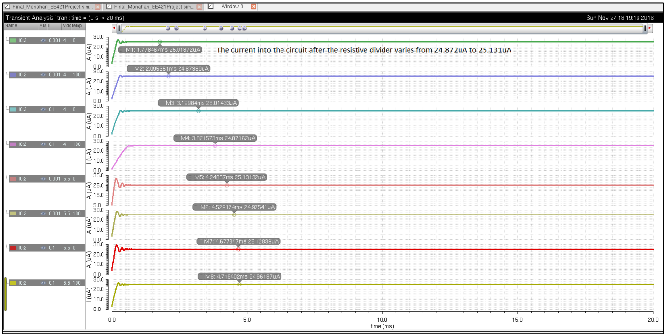
Figure 21 Current into comparator with varying VDD, current load and temperature.
