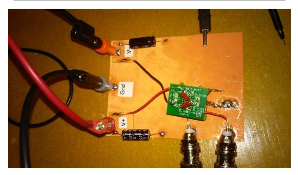
Testing of Passive 2<sup>nd</sup>-Order Sigma-Delta Modulator Circuit for Low-Power ADC
