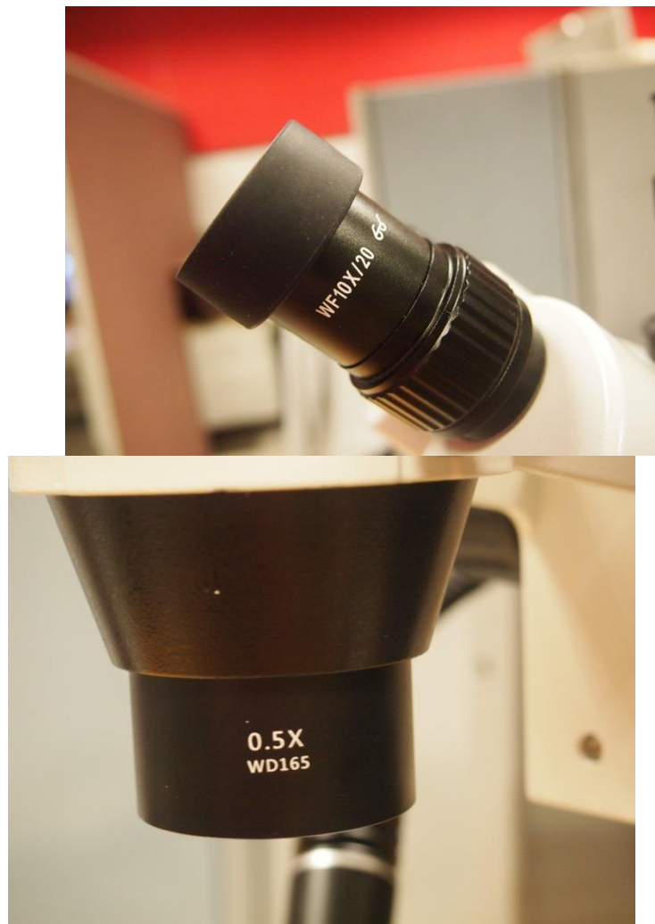
Figure 2 Eyepiece with 10X Magnification (top) and Objective Lens with 0.5X Magnification (bottom)
