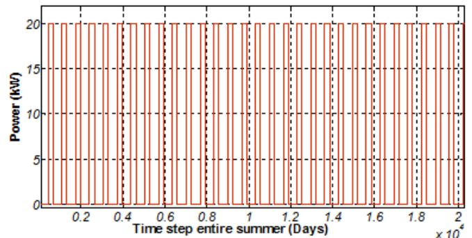
**Figure 7-** Constant 20kW produced based on 20.436kWh ESS1 for the whole summer.
