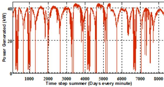
**Figure 5-** The CPV 7700 output pattern in kW, CER UNLV.
