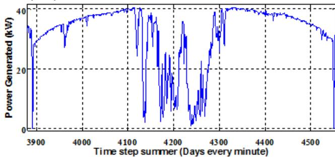
**Figure 3-** Typical power generation on a cloudy day.
