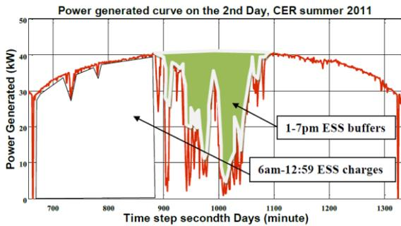
**Figure 6-** The ESS1 charges in the morning and buffers in the afternoon (Load shifting application).
