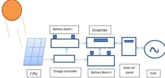
**Figure 4-** Grid-tied CPV with ESSs.
