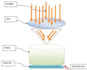
**Figure 1-** The optics of CPV.
