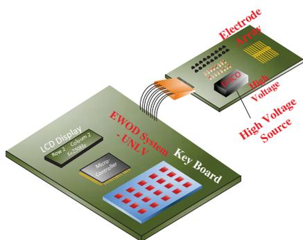
**Figure 3** – Diagram of the electro-wetting system.
