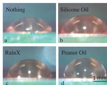
**Figure 5** – Differences in contact angles of pure water droplet on different coated Saran Wrap surfaces. No voltages applied. a. Nothing coated on the Saran Wrap; b. With silicone oil coated on the Saran Wrap. c. With RainX coated on the Saran Wrap. d. With Peanut Oil coated on the Saran Wrap.
