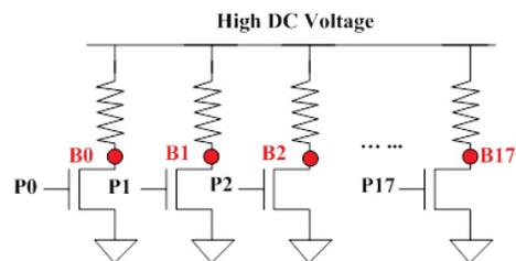
**Figure 1** – Schematic of the voltage supply circuit.
