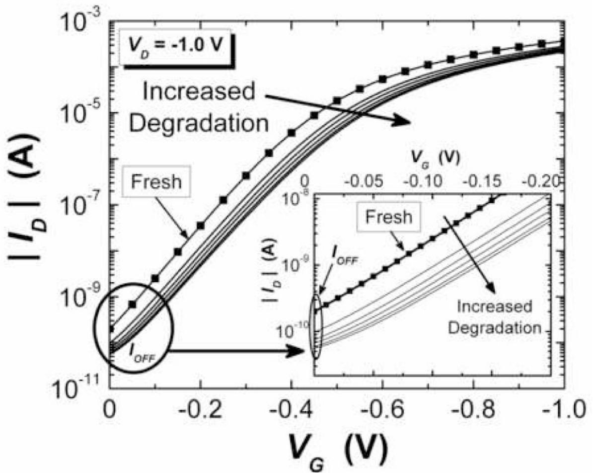
**Fig. 10.** Typical pMOSFET logarithm drain current ( $\log I_D$ ) versus gate voltage ( $V_G$ ) results for Fresh through stress cycle E, showing a decrease of approximately 82% in off-current ( $I_{OFF}$ ) after induced wear out. The  $I_{OFF}$  data is encircled and emphasized in the inset plot. Throughout the test, the drain voltage is held constant at -1V.
