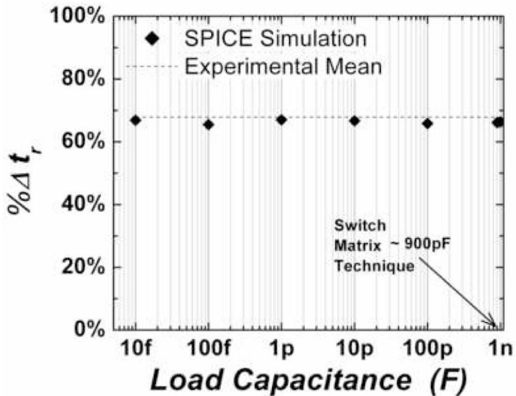
**Fig. 3.** SPICE simulation results showing  $\% \Delta t_r$  as a function of  $C_L$  for NAND circuit configuration 1-3 (Table I). Results indicate  $\% \Delta t_r$  remains fairly constant within the range of 10fF to 1nF. It is interesting to note that simulation results for  $\% \Delta t_r$  are near the mean value of experimental data obtained using the switch matrix technique. The arrow indicates the approximate  $C_L$  associated with the Switch Matrix Technique.
