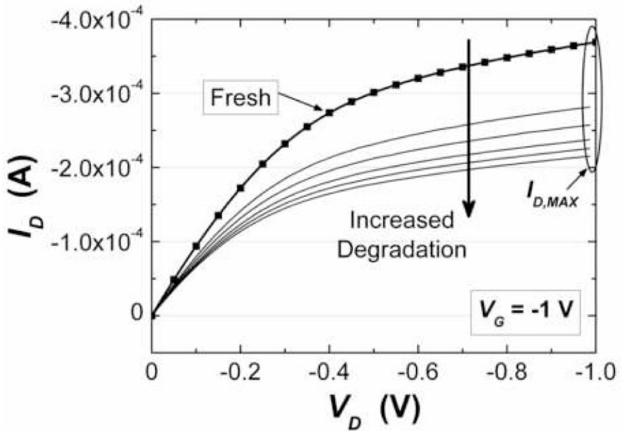
**Fig. 8.** Typical pMOSFET drain current versus drain voltage ( $I_D$ - $V_D$ ) results for Fresh through stress cycle E showing a decrease in  $I_{D,MAX}$  of approximately 43% with increasing wear out.  $I_{D,MAX}$  data is measured at  $V_D=V_{DD}$  (encircled). The gate voltage is held constant at -1 V throughout the test.
