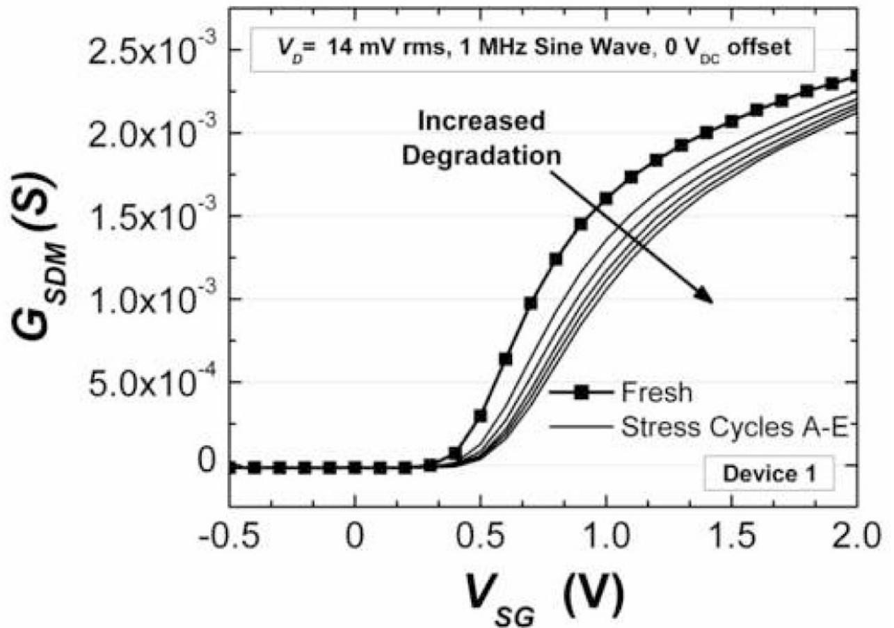
**Fig. 11.** Typical pMOSFET small-signal conductance measurement results for Fresh through stress cycle E showing a decrease of approximately 30% in source-to-drain conductance ( $g_{sdm}$ ) after induced wear out. The  $\% \Delta g_{sdm}$  results reported are measured at  $V_{SG} = V_{DD} = 1$  V. Throughout the test the drain voltage is held at a  $0V_{DC}$  bias with a  $14mV_{rms}$  sinusoidal signal at a frequency of 1MHz superimposed.
