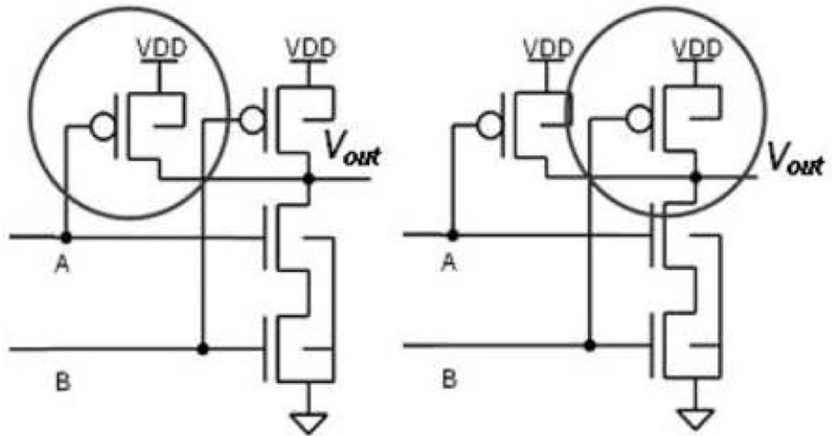
**Fig. 2.** NAND logic circuits illustrating position 1 and position 2 of the degraded pMOSFET. Following each stress cycle circuit characteristics were collected with the degraded pMOSFET in position 1 followed by collection of circuit characteristics with the degraded pMOSFET in position 2.
