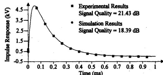
FIG. 4. The extracted impulse response with a disturbance SNR of 36.2 dB.
