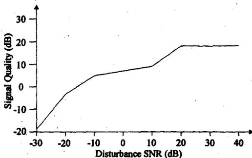
FIG. 6. Signal quality of the impulse response as a function of the disturbance SNR.
