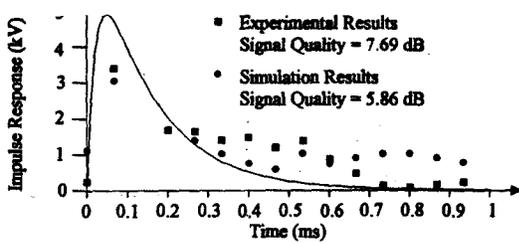
FIG. 5. The extracted impulse response with a disturbance SNR of 2.1 dB.
