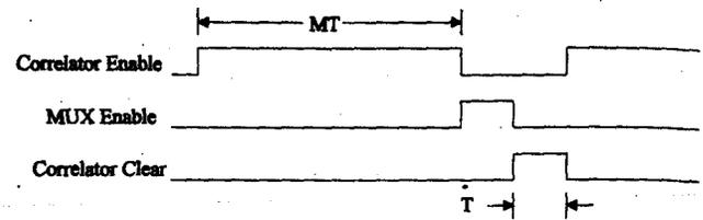
FIG. 7. The modified control signals used in the correlator.
