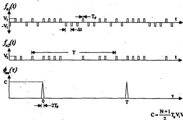
FIG. 2. The cross correlation of two unique  $m$ -sequence random impulse trains.
