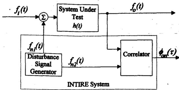
FIG. 1. Determination of a system impulse response using the cross-correlation method.
