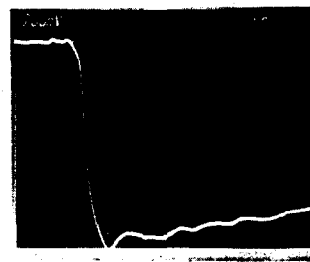
FIG. 3. Output of MOSFET pulser. 200 V/div and 5 ns/div.
